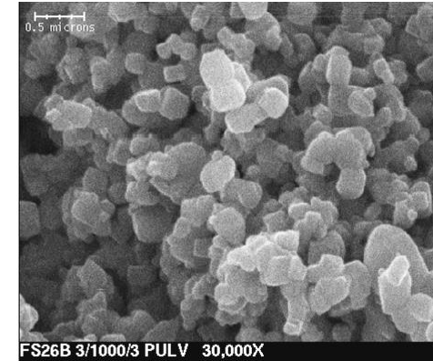
Conventional Calcine 1000 °C, 4 hr, D_s = 500 nm
