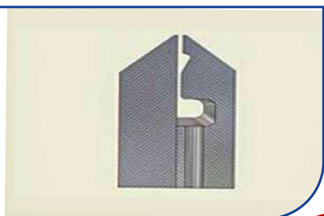
Slot Die section view displaying internal manifold
