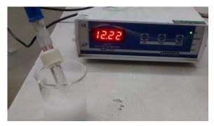
pH of Jarosite Slurry: 7 (Whole solution mentioned above in 700 ml of Jarosite)
