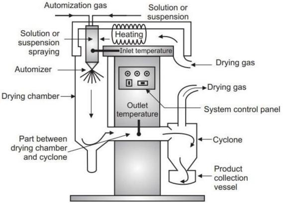
The diameter of the chamber is 2.5-9 meters and height 25 meters or more. An inlet for hot air is placed in the roof of the chamber and another inlet carrying spray disk atomizer is set in the roof. The spray disk atomizer is about 300 mm in diameter and rotates at a speed of 3000 to 50,000 r.p.m. Bottom of the dryer is connected to a cyclone separator.
