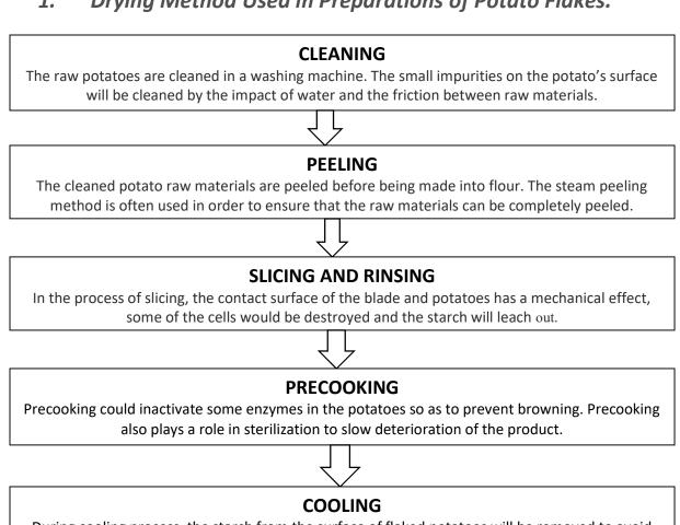
During cooling process, the starch from the surface of flaked potatoes will be removed to avoid caking during drying. The cooling will end only if the temperature in the middle of the flaked potatoes drops below 25 °C.
