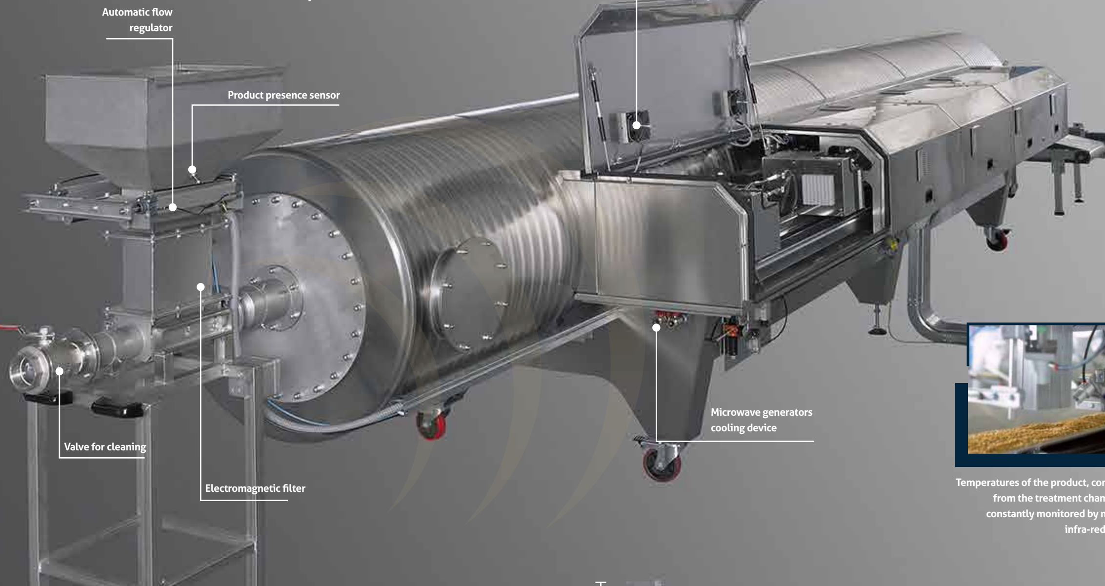
The product conveyance occurs by means of an helicoidal system
