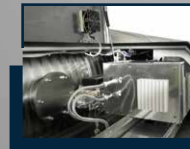
The device is endowed with six microwave generators, directly connected to the treatment chamber
