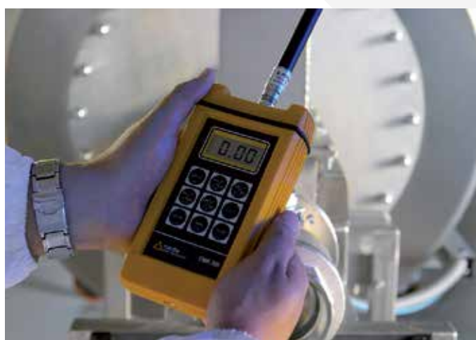
Isotropic sensor for measurement of the electromagnetic field in the area surrounding the device.
