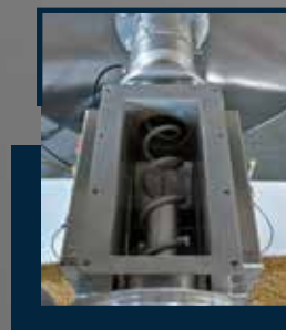
The product conveyance occurs by means of an helicoidal system
