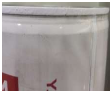
Touch-up Paint Applied Top Chime
